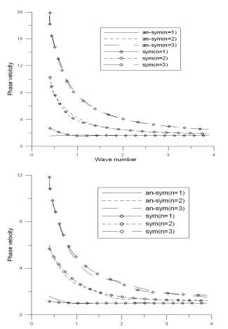
Fig. 1 Variation of phase velocity w.r.t wave number in mixture for symmetric and antisymmetric modes of propagation.
