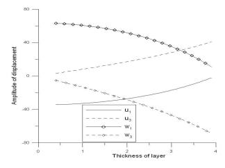
**Fig. 7** Variation of amplitudes of displacement components in mixture for symmetric mode.
