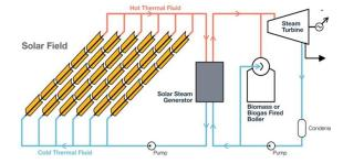
Fig. 3. Diagram of Biomass Solar Hybrid
