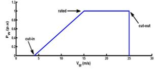
Fig. 2. Output power of wind turbine generators
