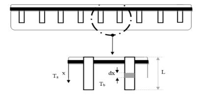
Figure 1. Geometry of a straight fin in solar air collector.
