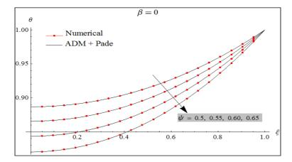
Figure 2. Temperature distribution in convective fins thermo-geometric fin parameter ( $\psi$ ) when  $\beta$ =0 With PADM method and Ns
