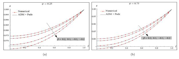
Figure 3. Temperature distribution in convective fins with variable thermal conductivity with PADM method and Ns
