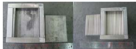
Fig. 2 Designed grooved die (right), flat die (left)
