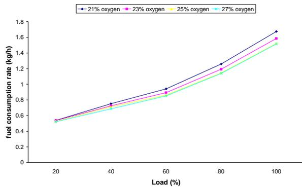
Fig. 2 Fuel consumption rate with load
