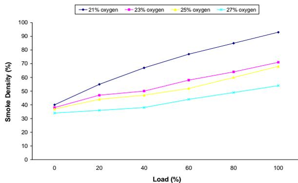
Fig. 5 Variation of Smoke Density with oxygen enrichment and load
