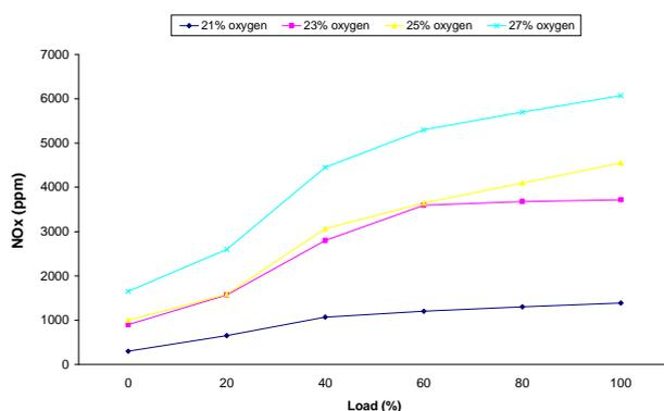
Fig. 6 Variation of NOx versus load for different oxygen enrichment levels
