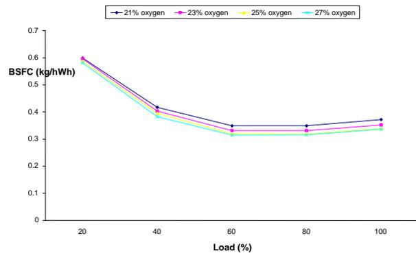
Fig. 3 Variation of BSFC with oxygen enrichment and load
