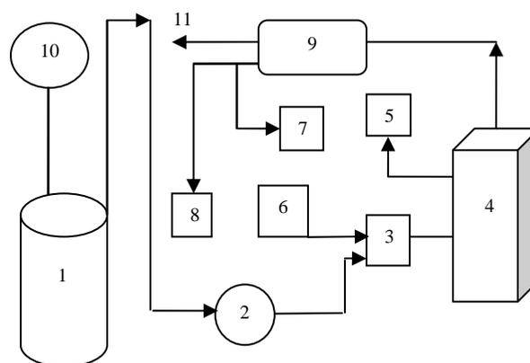
(1) Oxygen cylinder; (2) Gas flow meter; (3) Mixing chamber; (4) engine; (5) Exhaust gas thermometer; (6) Orifice meter; (7) NO<sub>x</sub> meter; (8) Smoke meter; (9) Exhaust; (10) Pressure gauge; and (11) to atmosphere
