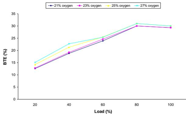
Fig. 4 Variation of Brake Thermal Efficiency with oxygen enrichment and load
