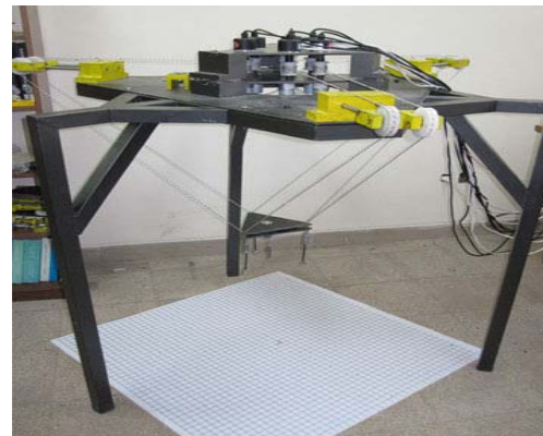
Fig. 9 Scheme of the designed IUST cable robot
