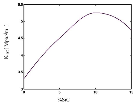
Fig. 3 Fracture toughness of nano composites vs. volume fraction of SiC
