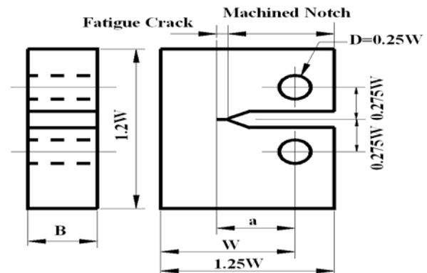
Fig. 1 Size of specimens based on ASTM standard [6]
