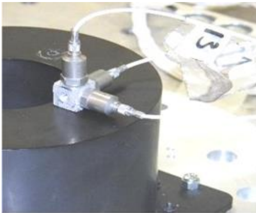
Fig. 5 Tri- directional vibration sensor random test on a satellite battery pack
