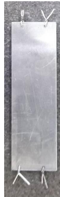
Fig. 3 The sample fastened by steel wires before the rolling process.
