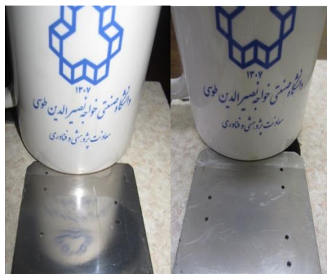
Fig. 13 Effect of MAF process on IN718 surface quality
