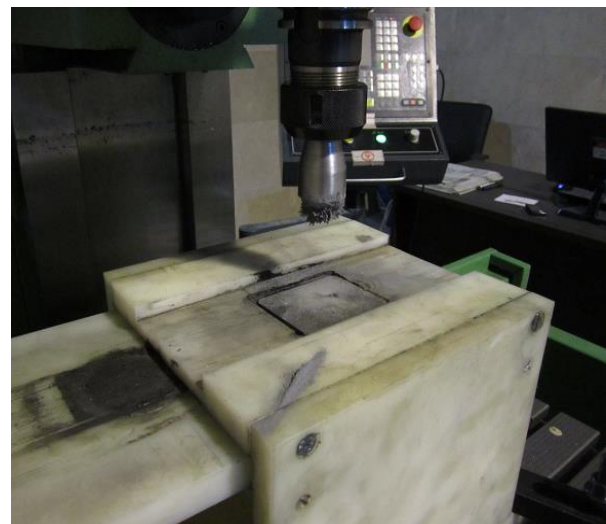
Fig. 4 Magnetic Abrasive Finishing process on IN718 surface
