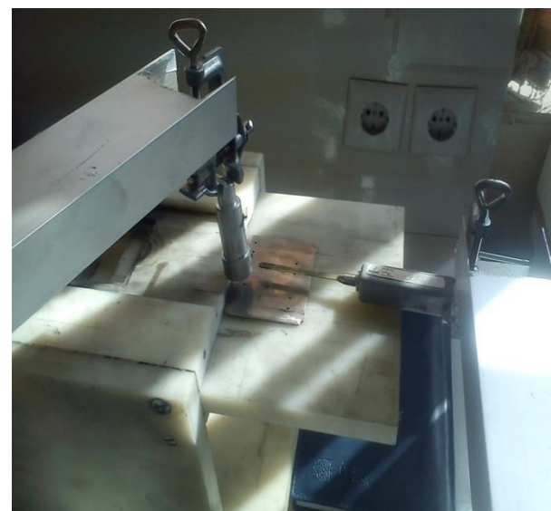
Fig. 1 Measuring procedure of magnetic flux density (mT) using gauss meter
