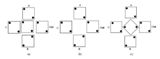
Fig. 2 Faults of majority gate, (a) misalignment cell, (b) missing cell, and (c) dislocation cell.
