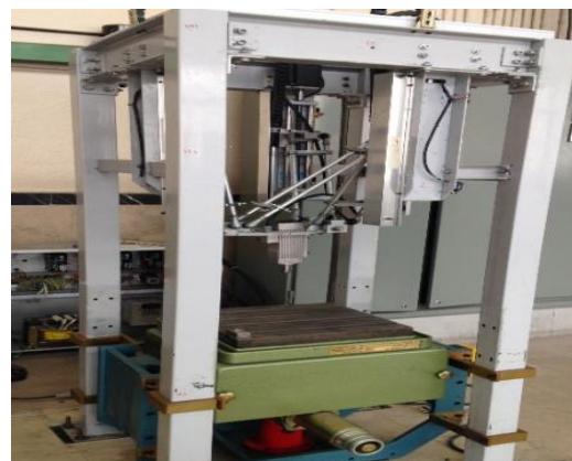
Fig. 1 2-PR(Pa)U-2-PR(Pa)R parallel mechanism with 4 degrees of freedom
