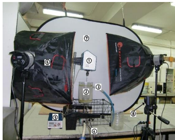
Fig. 2 Mixer laboratory scale setup (1: mixer, 2: mixer vessel 3: outlet, 4: organic and aqueous inlets, 5: mixer controller 6: flash projector, 7: reflecting surface)
