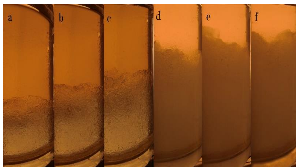
Fig. 9 Mixing region and flow hydrodynamics in impeller speed of 150 rpm, a) clearance of 5 cm b) clearance of 6 cm c) clearance of 7 cm d) clearance of 8 cm e) clearance of 9 cm e) clearance of 10 cm
