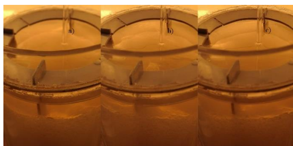
Fig. 6 Turbulence around baffle for 3 different impellers a) PTU, b) RT, c) PTD
