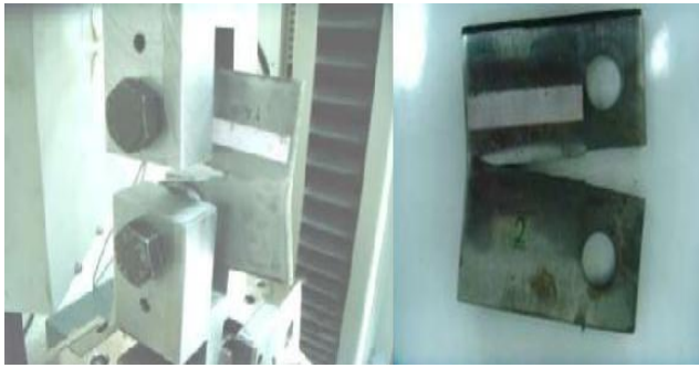
Fig.9 Specimens on test machine and after test.
