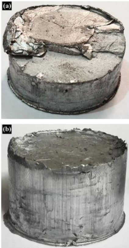
Fig. 3 Cold pressed samples under 400 MPa pressure; (a) without keeping the pressure for specific time duration, (b) keeping the pressure for 5 minutes
