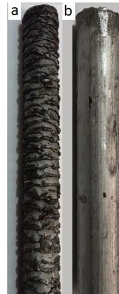
Fig. 4 Effect of suitbale lubrication on surface quality of hot extruded Al-3 vol% SiC nanocomposites; (a) Without lubrication, (b) With lubrication
