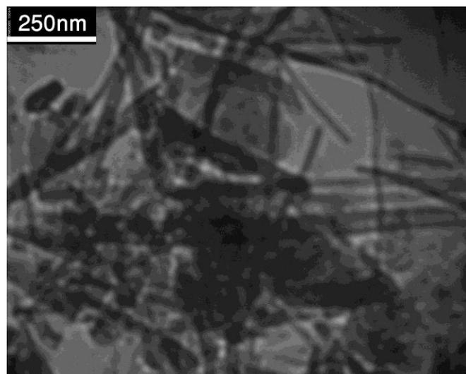
Figure 6. TEM micrograph of m-CMC-PAMH nanocomposite hydrogel (20% m-MMT).
