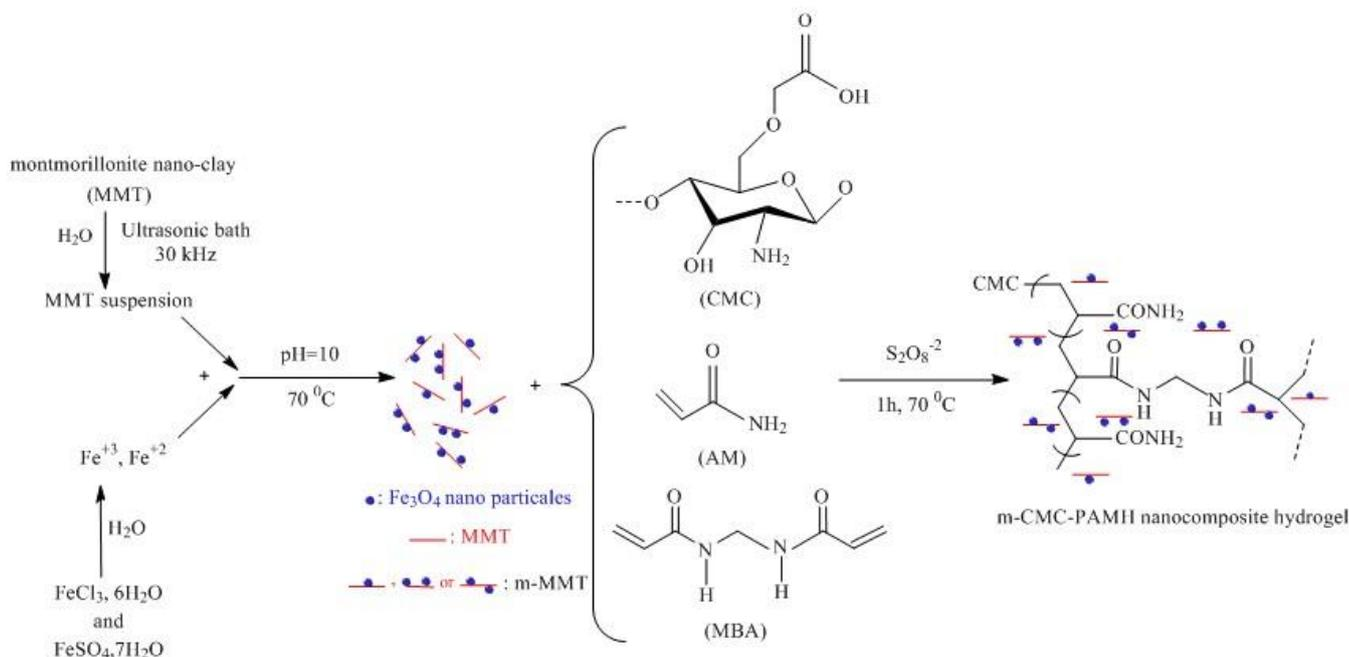
**Figure 2.** Scheme for the preparation procedure to proposed adsorbent of m-CMC-PAMH nanocomposite hydrogel.
