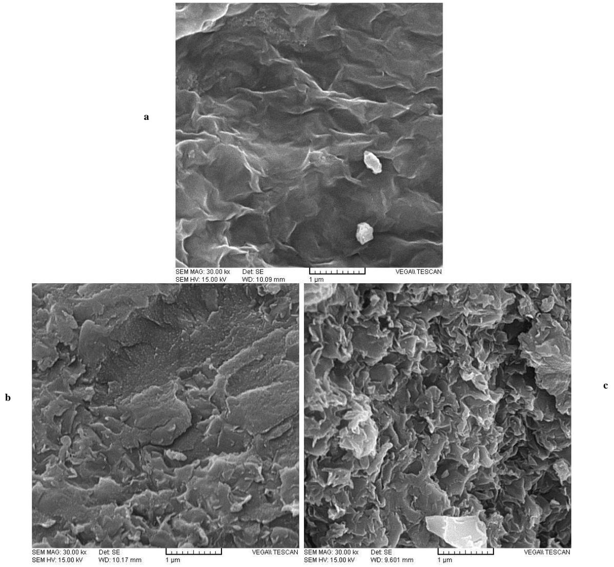
Figure 5. SEM images of (a) CMC-PAMH, (b) m-CMC-PAMH (10% m-MMT) and (c) m-CMC-PAMH (20% m-MMT).
