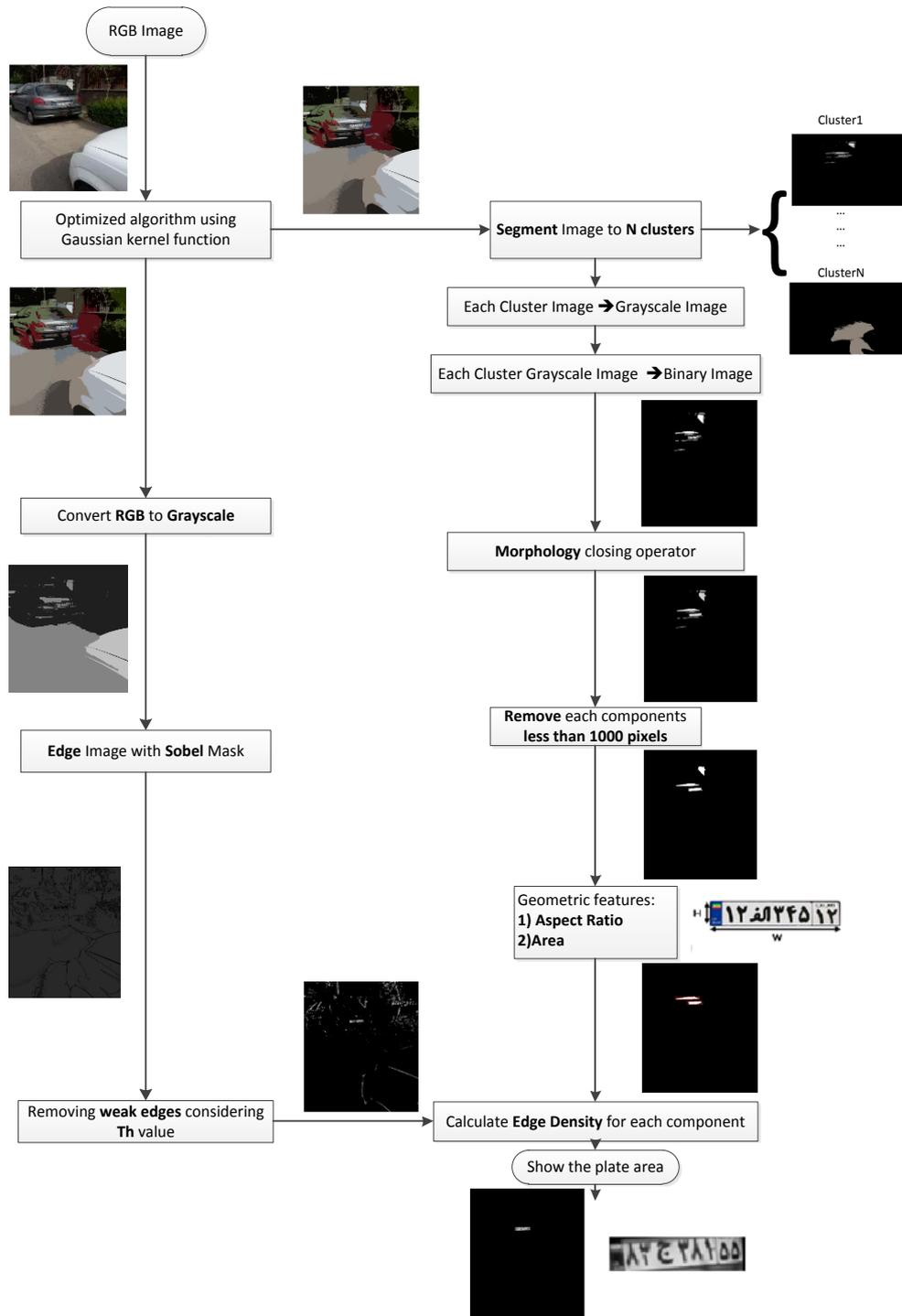
Fig. 2. Block Diagram of the optimized MS algorithm for Iranian license plate detection.
