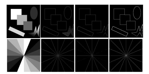
Figure 7. Original image, canny edge, Sobel edge, new detector
