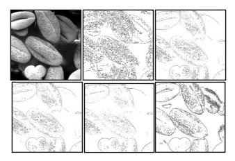
Figure 6. Edge map: Original image, canny edge, Sobel edge, Roberts's edge, Perwit edge, new detector
