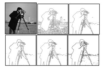
Figure 5. Edge map: Cameraman image, canny edge, Sobel edge, Roberts's edge, Perwit edge, new detector
