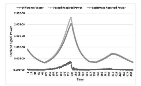
Figure 13. Scenario3: Diagram of the received legitimate signal power vector, the received forged signal power vector, the difference vector between the received legitimate and forged signals
