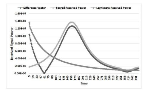
Figure 5. Scenario 1: Diagram of the received legitimate signal power, the received forged signal power and the difference vector between the received legitimate and forged signals
