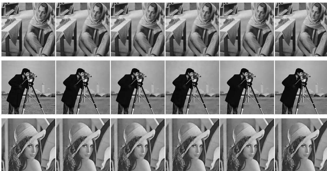
Figure 5. From left to right: Original image, result of denoising of noisy images with noise standard deviation 20 by NLM [6], NLM- C_p [24], NLM-SAP [15], NLM-PCA [11] and Proposed method (VPID). From top to bottom: Barbara, Cameraman and Lena images.
