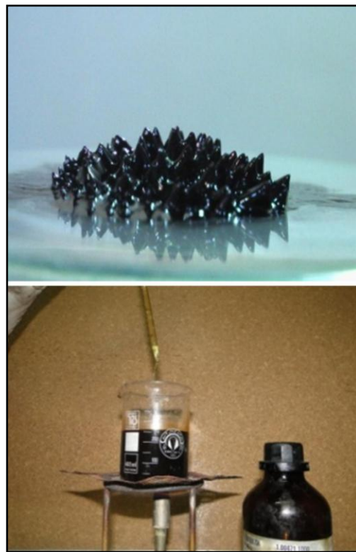
Fig. 1. Ferrofluid based on hydraulic oil
