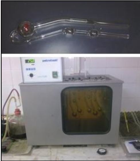
Fig. 2. Cannon-Fenske viscometer and the oil bath
