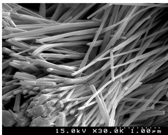
Figure 4: TEM image of \text{Sb}_2\text{Se}_3 nanorods.
