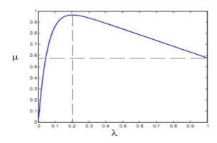
Figure 1. Dependence of friction coefficient on slip ratio
