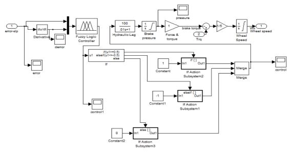
Figure 2. Obtaining final control signal
