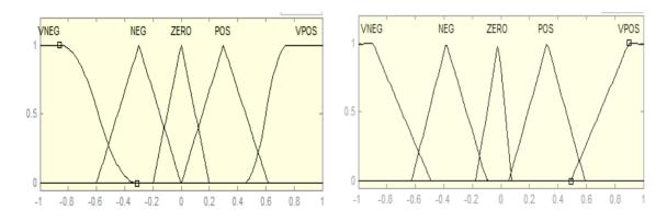
Figure 3. membership functions of input variables
