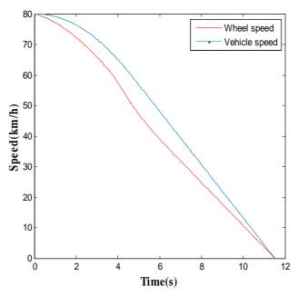
Figure 13. Wheel and vehicle speed for dry road
