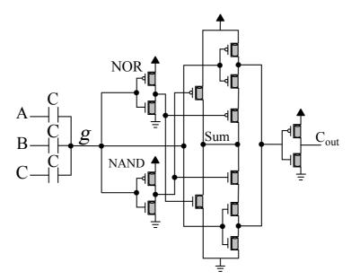
Figure 3. The schematic of FA1 [13]
