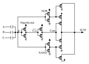
Figure 5. The schematic of SyMuT [15]
