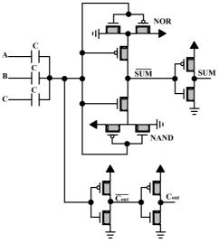
Figure 4. The schematic of FA2 [14]
