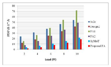
Figure 9. PDP versus output load
