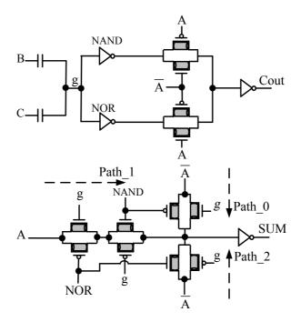
Figure 6. The schematic of the proposed full adder
