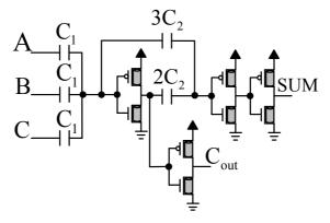
Figure 2. The schematic of 3c2c [12]
