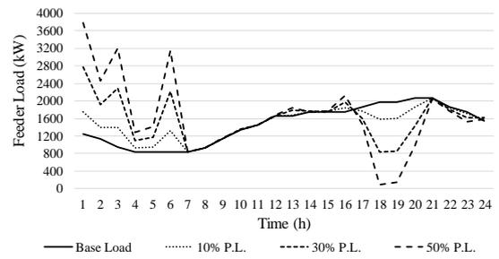
Fig. 7. Feeder load demand in case 2.
