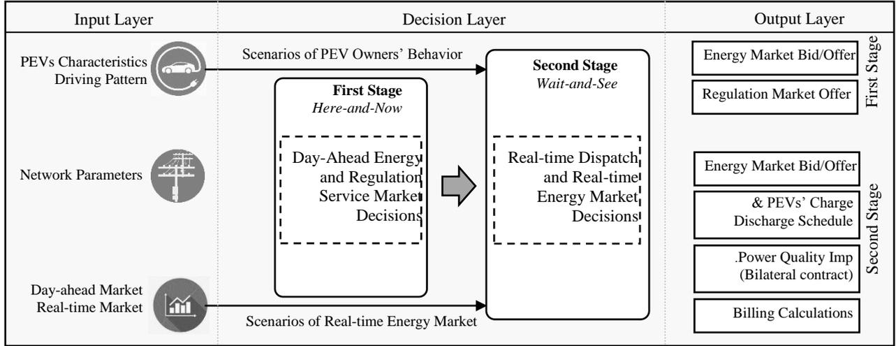
Fig. 2. Schematic of the proposed two-stage stochastic model from the aggregator's perspective.
