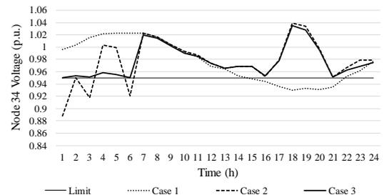
Fig. 11. Daily voltage curve of node 34 for 50% Penetration Level.
