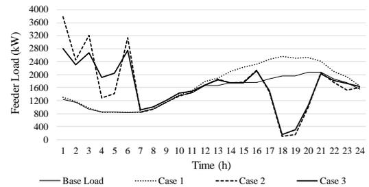
Fig. 10. Feeder load demand for 50% penetration level.
