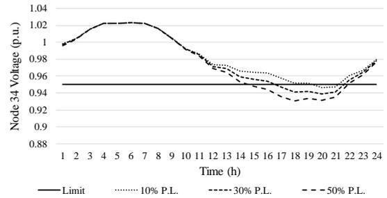
Fig. 8. Daily voltage curve of node 34 in case 1.
