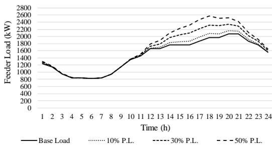
Fig. 6. Feeder load demand in case 1.
