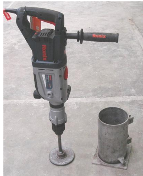
Figure 2. Roller Compacted Concrete condenser view
