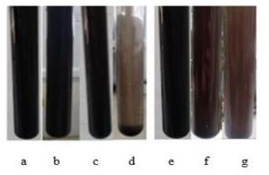
Fig. 2. TEG-water based nanofluid contained TX-100 at the first day (a), TX-100 is still stable at the next day (b), TX-100 is still stable during a 10-day period (c) and TX-100 within two weeks (d). Pure TEG based nanofluid contained TEAOH on the first day (e), on the next day (f) and is still stable during a 3-day period (g).
