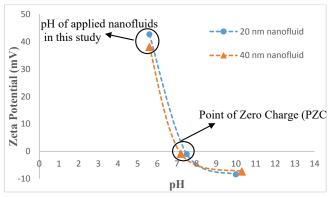
Fig. 3. Effects of pH on the zeta potential of TEG-water based nanofluids.
