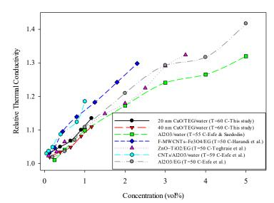
Fig. 14. Experimental data at 60 °C compared to other experimental studies in the literature using KD<sub>2</sub> pro thermal analyzer at various concentrations [57-61].
