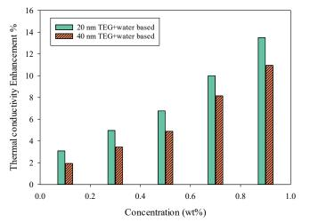
Fig. 8. Thermal conductivity enhancement for various nanofluid concentrations at 60 °C.
