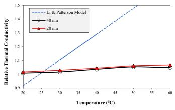
Fig. 12. Relative thermal conductivity for 0.5 wt.% nanofluids compared with Li & Peterson model.
