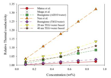
Fig. 13. Experimental data at 60 °C compared to empirical correlations at various concentrations.
