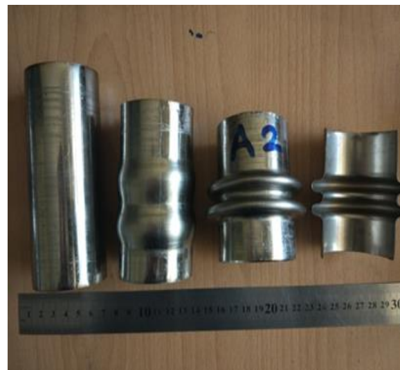
Fig. 1 Various steps of hydroforming process in order to manufacture a bellows from an initial cylindrical tube (From left to right of picture)
