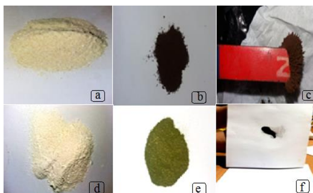
Fig. 2. (a) Pretreated Egg shell, (b) MNLES, and (c) MNLES totally attracted to magnet, (d) pretreated Egg membrane, (e) MNLEM, and (f) MNLEM totally attracted to magnet.
