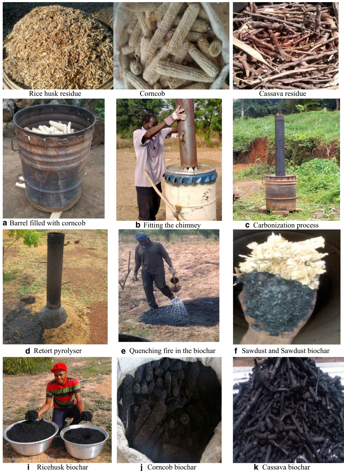
Fig. 1 Biochar production from selected crop wastes using the Elsa pyrolysis barrel. Source: Billa et al. (2017)
