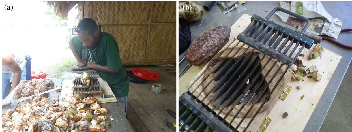
Fig. 1 a Locally designed cocoa pod dicing contraption; b dicing action between blades placed at 2 cm apart
