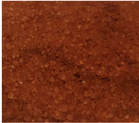
Fig. 5 Sand after bioclogging with iron-based biogROUT
