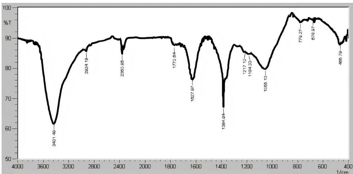
Fig. 3. FTIR SPECTRA OF the biosynthesized SMSE-AgNPs.
