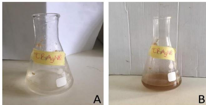
Fig. 1. Synthesis of the AgNPs (a) 0 min after the addition of the plant extract to the silver nitrate (b) Formation of deep brown colouration after 30 min.
