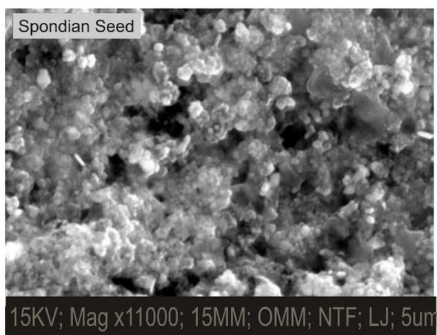
Fig. 6. FESEM ANALYSIS of the biosynthesized SMSE-AgNPs.
