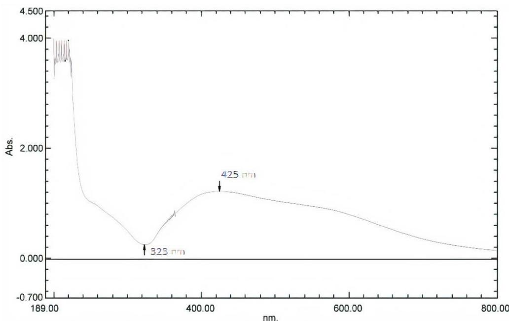
Fig. 2. The UV-Visible spectrum of the biosynthesized SMSE-AgNPs.
