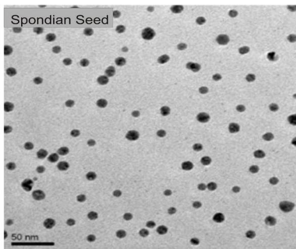
Fig. 4. TEM ANALYSIS of the biosynthesized SMSE-AgNPs.
