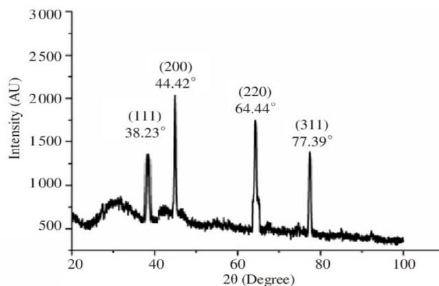
Fig. 7. XRD SPECTRA of the biosynthesized SMSE-AgNPs.
