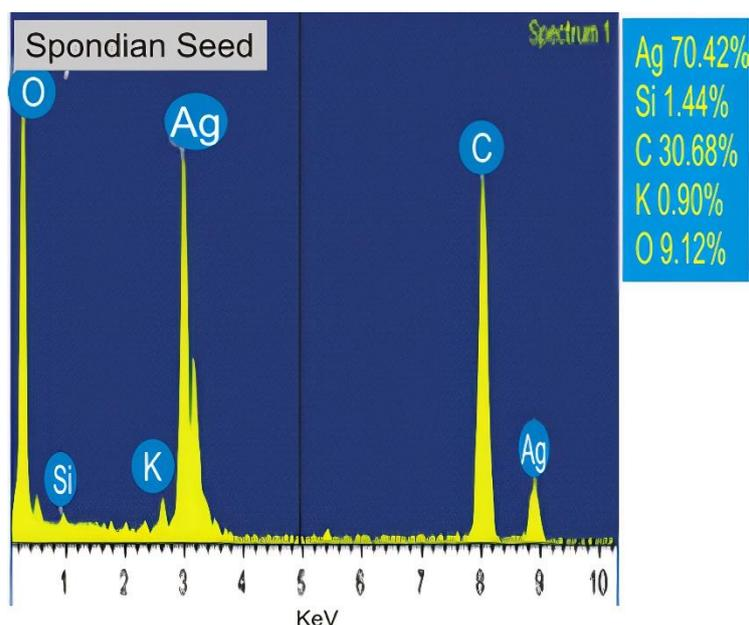
Fig. 5. EDX SPECTRA of the biosynthesized SMSE-AgNPs.
