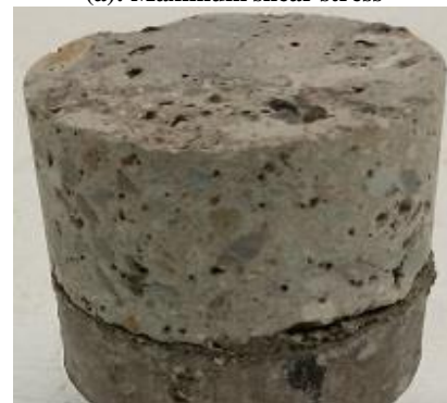
(b): Failure at common boundary
