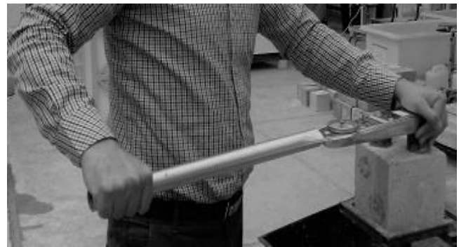
(b) Mechanical properties Fig. 3 Performing the "twist-off" test.
