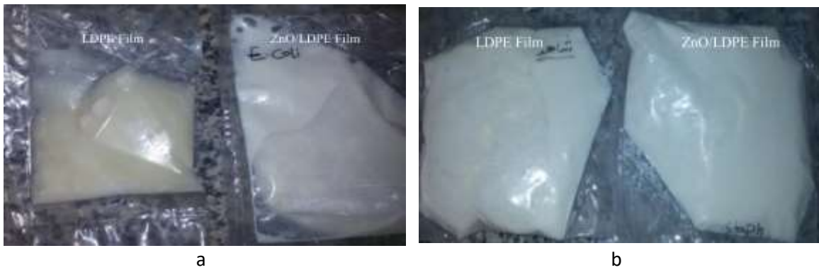
Fig. 5. Milk sample contain a) E. coli and b) S. aureus packaged into LDPE and ZnO/LDPE films.
