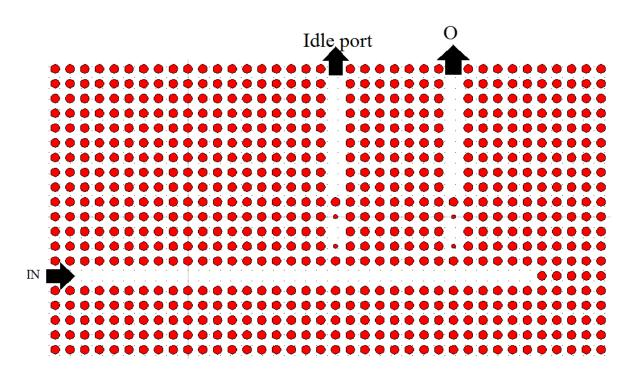
Fig.6. The optical FSK demodulator.
