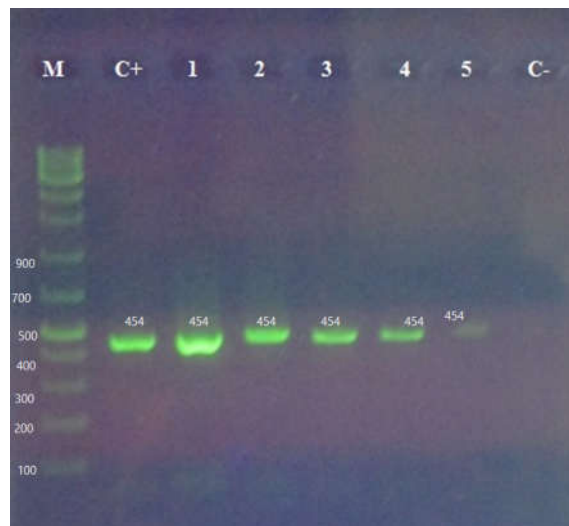
Figure 3: detection limit of the optimized PCR test. M: DNA Ladder (bioflux) marker size 1Kb. C+: (positive control) 454 bp PCR product from Herpes Simplex Virus I. 1: 500,000 DNA/Reaction. 2: 50000 DNA/Reaction. 3: 5000 DNA/Reaction. 4: 500 DNA/Reaction. 5: 50 DNA/Reaction. C-: negative control.
