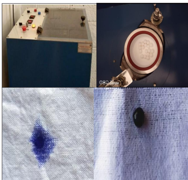
Fig. 1. Milling process of TiO 2 and water repellency of untreated & TiO 2 treated cotton fabric.
