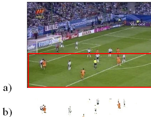
Fig. 6. The player gathering detection by using player detection on the grass specific area and by using a threshold on the non-grass pixel count
