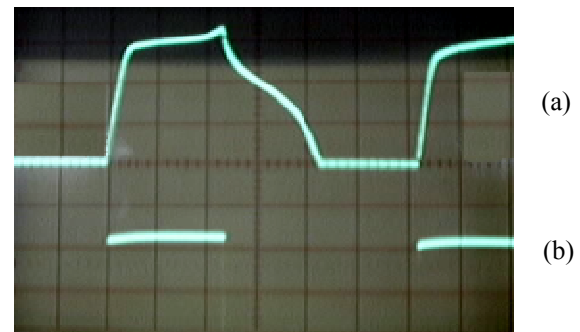
Fig. 12. a) Actual current waveforms for 5 Deg. of the advancement b) Power switches turn on time duration
