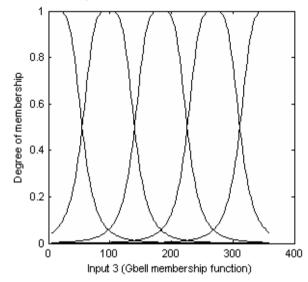
Fig. 5. The inverted input membership functions of rotation angle of the first motor.
