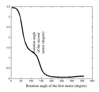
Fig. 9. The Rotation angle of the second motor versus Rotation angle of the first motor.
