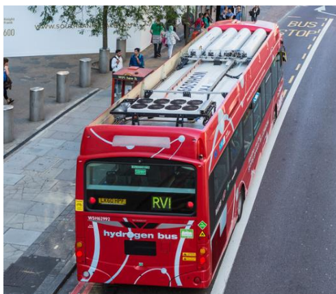
Fig. 2. Rooftop hydrogen storage on the FCETBs (source Sealord photography on Smugmug).
