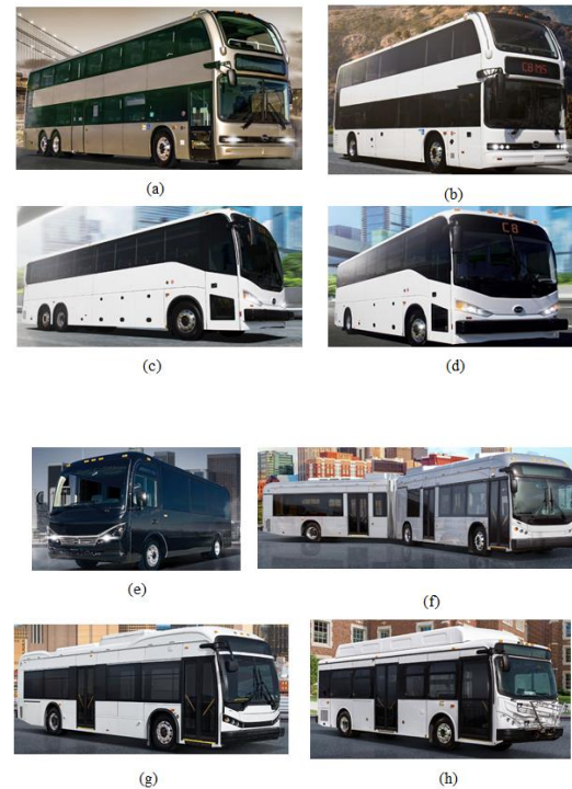
Fig. 5. Photographs of BYD bus models a) 45' double decker electric bus b) 35' double decker electric bus c) 40' electric motor coach d) 35' electric motor coach e) 23' electric motor coach f) 60' electric transit bus g) 35' electric transit bus h) 30' electric transit bus (source: en. BYD.com)
