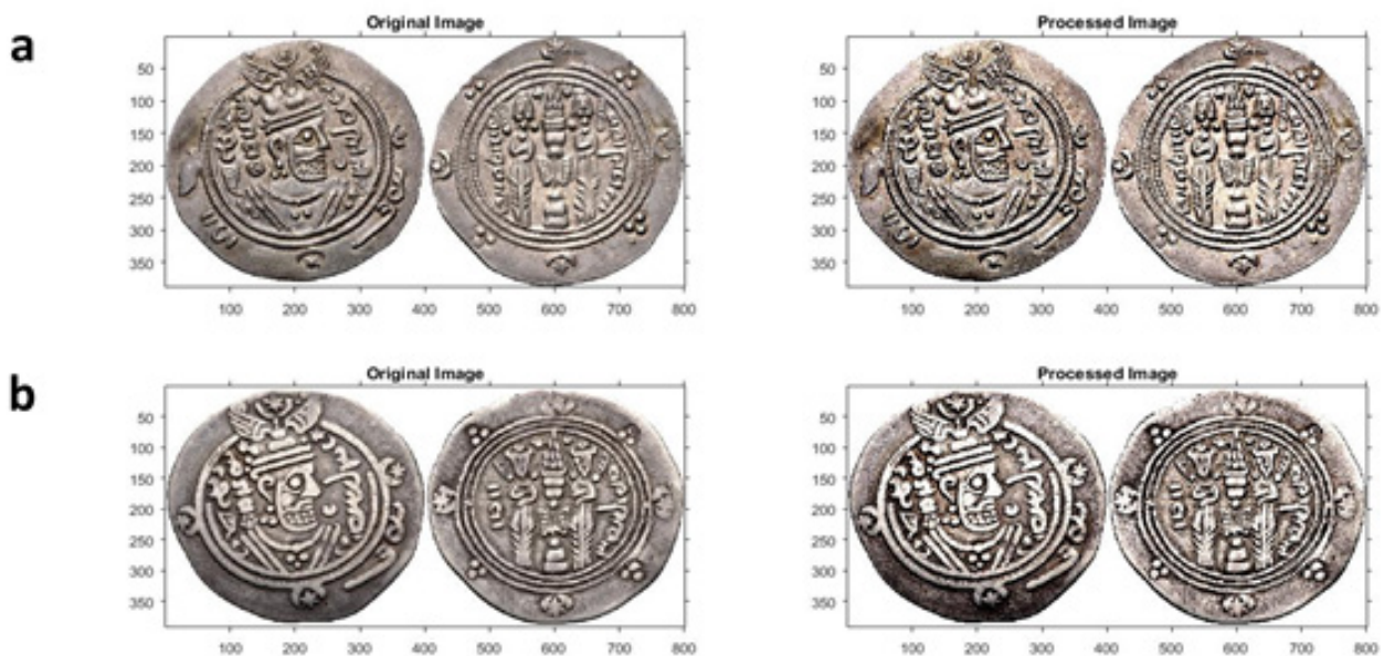
Fig. 7: Unsharp masking filter on the coin image, a) image of Farkhan the Great, b) image of Khursheed Daboui
