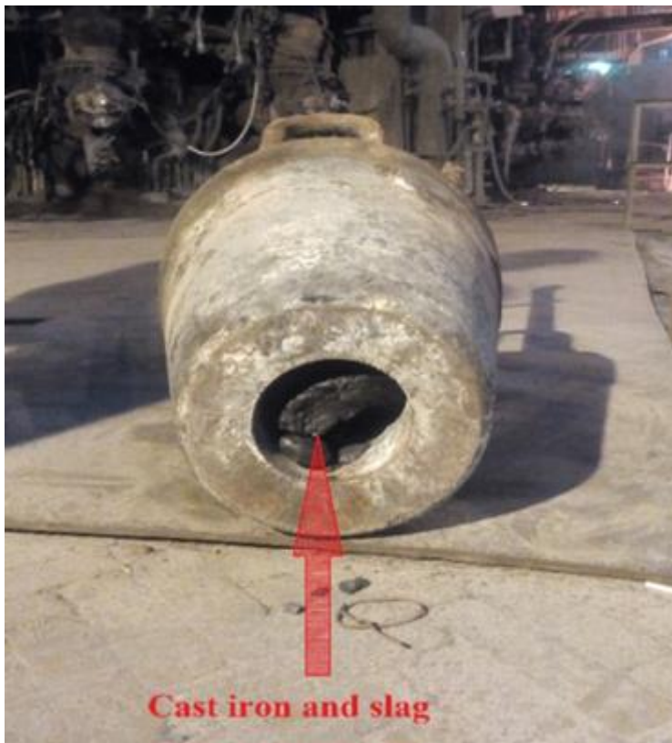
Figure 19. Newly developed tuyere with AZ coating after the blast air passage filled up with the melt and removal from the blast furnace
