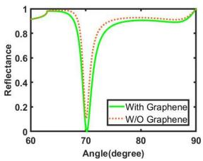
Fig. 6 The reflection spectrum of the biosensor with/without the graphene layer
