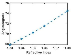
Fig. **4** The curve of biomaterial refractive index changes according to resonance angle.
