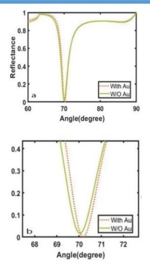
Fig. 7 a) The reflection spectrum of the biosensor with/without gold layer. b) magnification of the dip curve.
