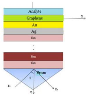
Fig. 1 Schematic view of proposed biosensor
