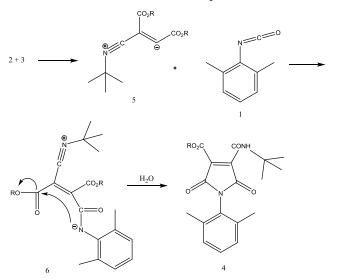
Scheme 2: The plausible mechanism for the synthesis of pyrrole derivatives.
