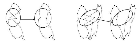
Figure 6. 1-1 Exchange mover for single route (left) and for multiple routes (right)
