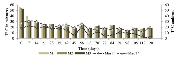
Fig. 1 Temperature profile of the mixtures M1, M2 and M3 during compost stage
