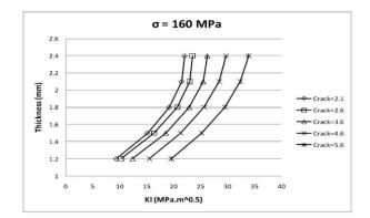
Stress intensity factor along the thickness for different cracks (loading 160 MPa).
