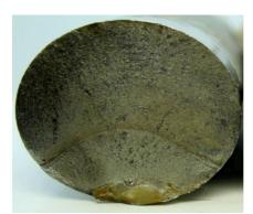
Many components of aerospace structures are subject to fatigue loading. There are many different criteria for predicting fatigue life. Fig. (1) shows a sample of the failure of a rod due to fatigue crack growth:
