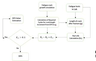
**Fig.2** Extrapolation method for EIFS calculation.
